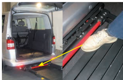
Toe protection bar with micro-switched operation cut-out
