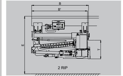
Side fitting for rigid vehicle - 2 folds platform
