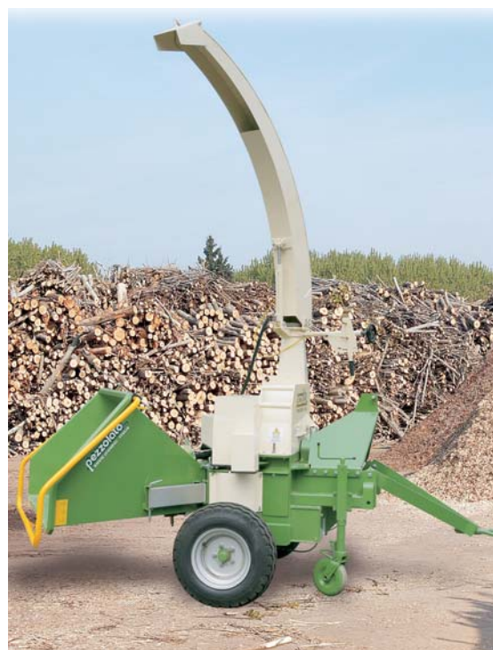
Chipping machine for chips heating system H 980/300 with extended output conveyor, equipped by hydraulic movements for deflector lifting, rotation and orientation
