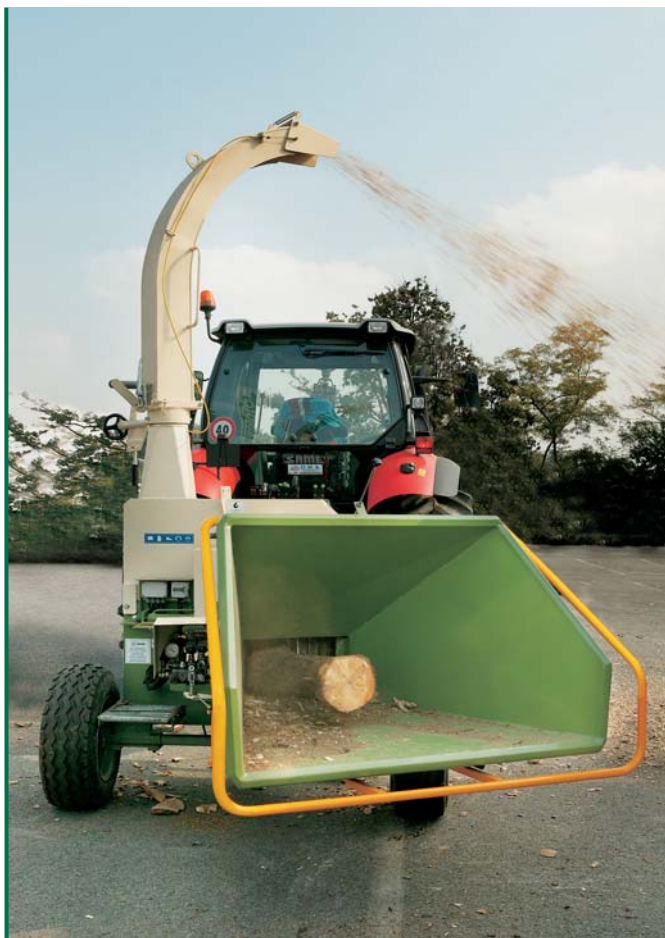
Chipping machine H 880/250 can chip logs up to 25 cm of diameter.
