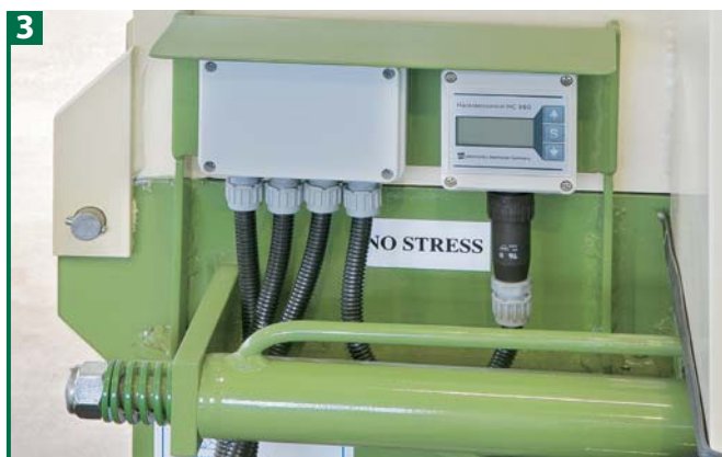
The electronic "no stress" device adjusts feeding of the material to be chipped, in relation to the power available, eliminating wearing forces.
