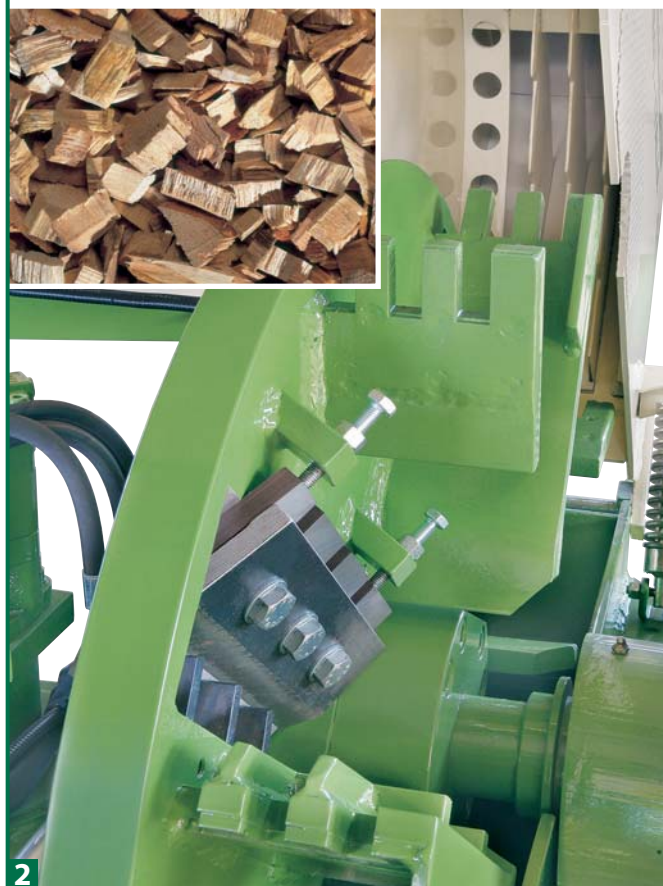
Detail of the material feeding mouth; the feeding rollers are visible on the base and, in the background, the disc with a chipping knife. Roller speed can be adjusted by the operator, in relation to the type of material to be chipped.
