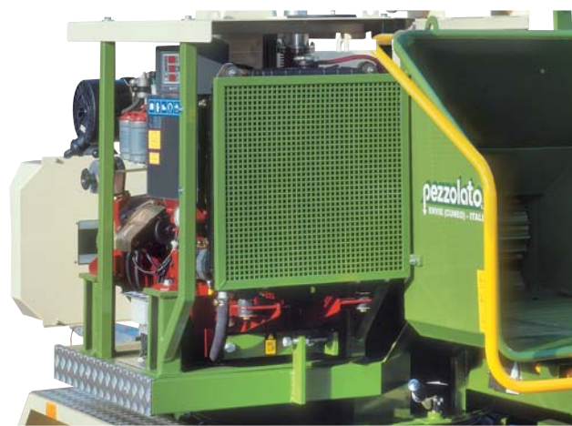
The lateral motor, as well as making the structure compact, simplifies inspection and maintenance activities.
