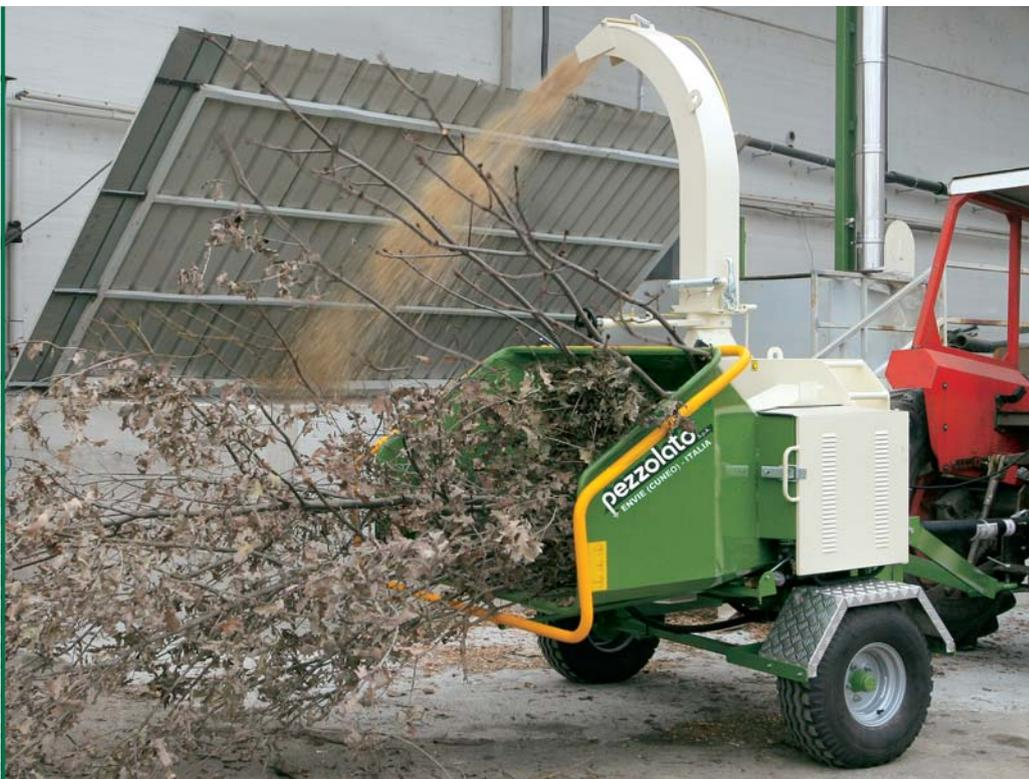
*PZ 250 G at work, mounted on trailer for low speed transport. This version has a 3-point hitch and support feet.*
