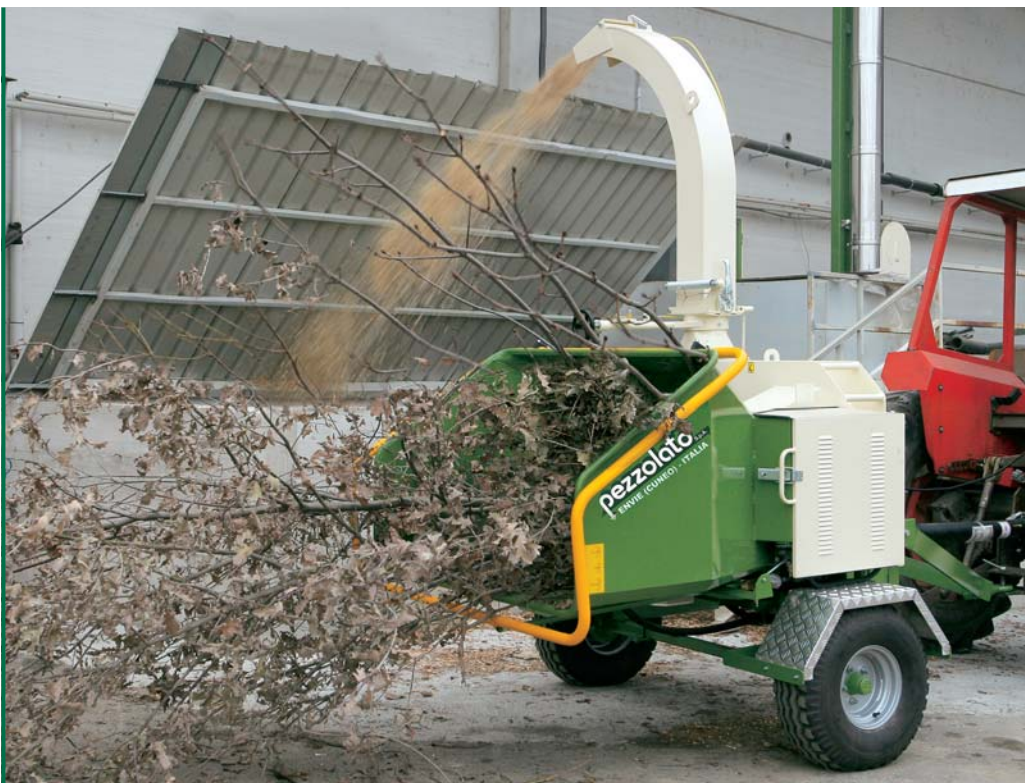
PZ 250 G at work, mounted on trailer for low speed transport. This version has a 3-point hitch and support feet.
